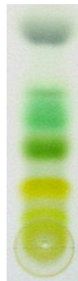
Thin layer chromatography is used to separate components of a plant extract, illustrating the experiment with plant pigments that gave chromatography its name
