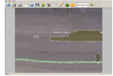
Figure 3. Lane marking and road defects are mapped with a minor user interaction.
